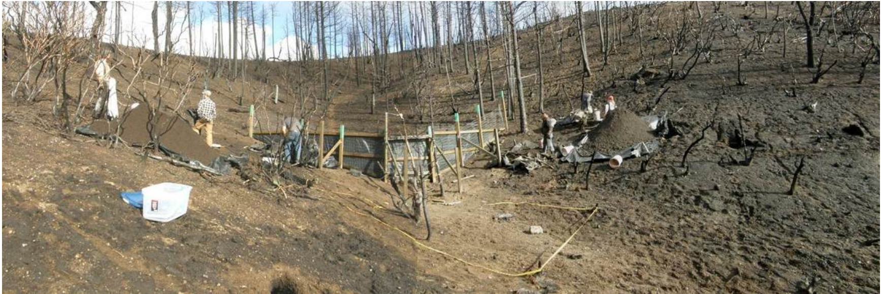
Figure ES-6. This photograph is looking upslope during a sediment fence cleanout of a control site. Note the people for scale. Sediment has been removed from within the sediment fence, weighed, and then piled on the sides and downslope of the sediment fence. As a control site, this swale received no salvage logging nor contour subsoiling. Note that on the control sites rill erosion features began forming on the burned hill slopes immediately after rainfall events. At this control site a main channel has begun to form; it shows as the lighter brown streak extending uphill from the fence through the middle of the swale. The sediment pictured accumulated during the first 3 months following fire containment.
