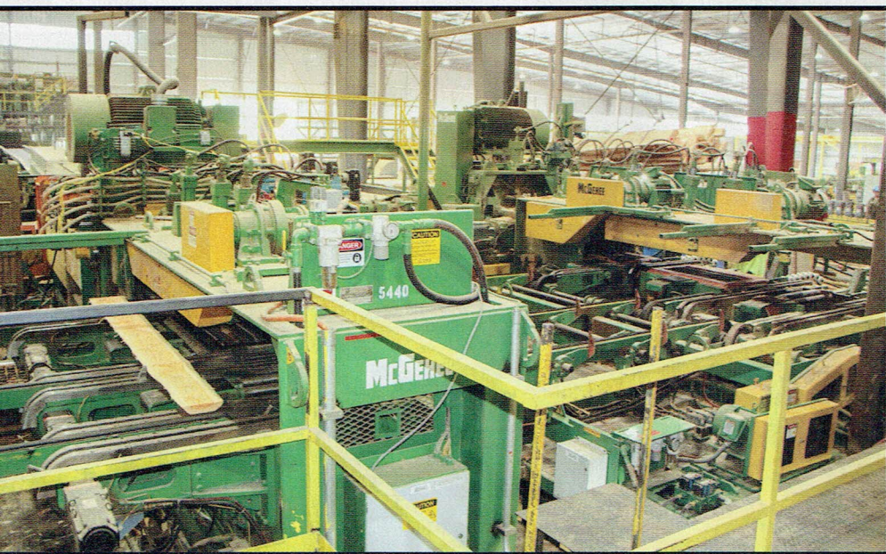
Off-line gang, edger and resaw handle any boards that need additional processing.
