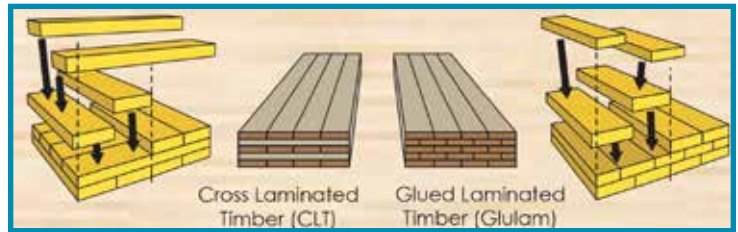
Illustration of how two popular mass timber products, CLT and glulam, are made. Source: https://www.researchgate.net
